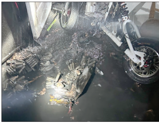
A lithium-ion battery from an electric bicycle exploded in a Holyoke apartment causing serious injuries to a resident. The battery’s remnants and debris are pictured here. Submitted photo
